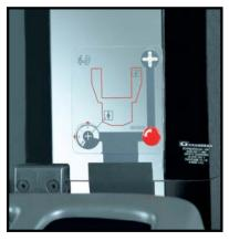
Heads-up display. For quick reference, Raymond's heads-up display indicates 4-D travel direction. Mode indicator lights make four-directional selection and automatic positioning easy.
