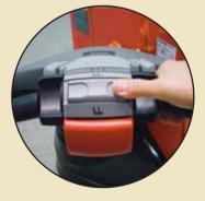
**To optimize load handling**, the RAS handle contains proportional lift lower for smooth, fine positioning of loads.
