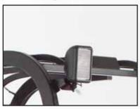
Certain load handling situations require more light than that provided by existing warehouse lighting systems. Work area lights are normally mounted in pairs, providing light to illuminate dimly-lit storage areas. As a consequence, work lights may thereby reduce operator eyestrain and increase productivity. The lights are individually adjustable by the operator to the application requirements.
