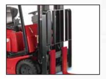
In certain environments of use, high palletized loads or loads stacked higher than the height of the carriage must be handled. The load backrest is an extension of the carriage height and serves to stabilize and provide additional support for such loads. As a consequence, the expanded load backrest extension assists in preventing material from falling and reduces load damage.
